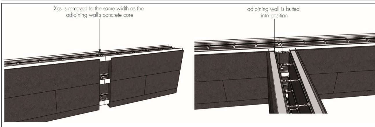
Figure 8 T-junctions in formwork
